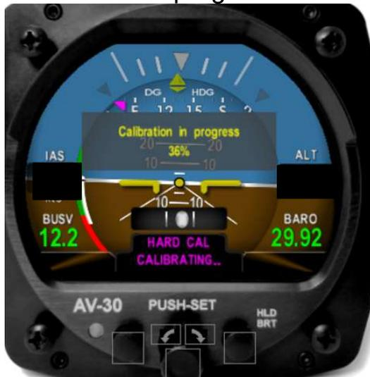
8. AV-30 will indicate "Calibration successfully completed Press DONE" Press the left button under "DONE" and the calibration will be complete. If an error is shown, repeat the calibration process.
